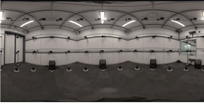
Fig. 2: Equirectangular photo of one of the loudspeaker arrays built for the IAP. (Photo credit: Scott Colburn)
