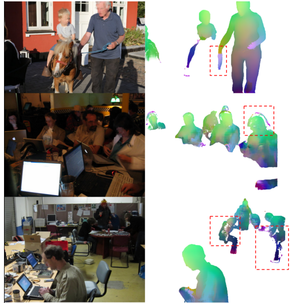
Figure 5. Failure cases. Most failure cases happen for low resolution images with occlusions and/or bad lighting.
