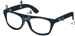
Fig. 3. Illustration of the microphone array mounted on glasses with the approximate microphone positions.
