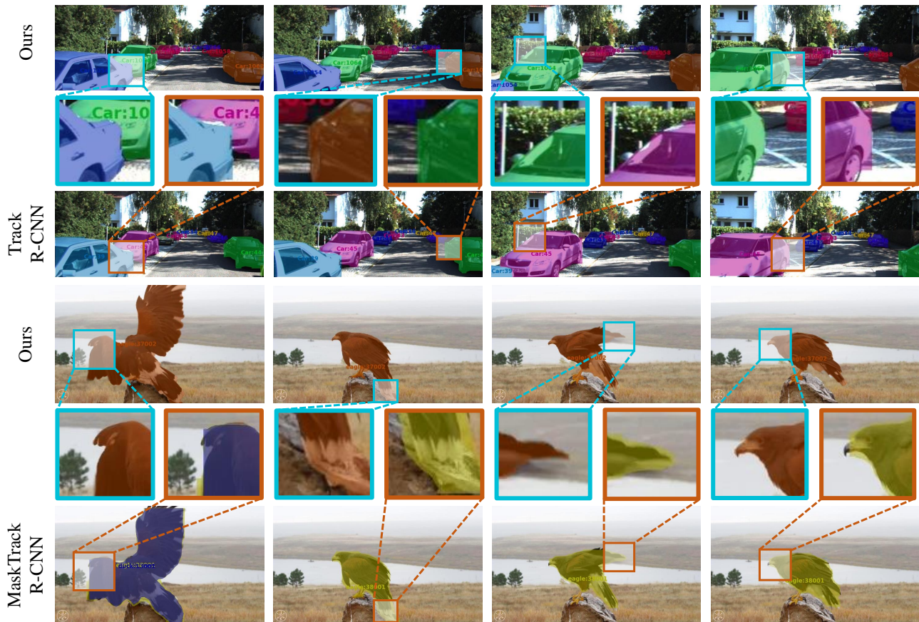
Fig. 5. Qualitative results of our STC-Seg in comparison with TrackR-CNN [10] and MaskTrack R-CNN [11] on KITTI MOTS and YT-VIS respectively. All compared methods use ResNet-101 with FPN.
