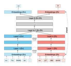
Figure 1: On the impact of anchor points and parameter sharing on the emergence of multilingual representations. We train bilingual masked language models and remove parameter sharing for the embedding layers and first few Transformers layers to probe the impact of anchor points and shared structure on cross-lingual transfer.
