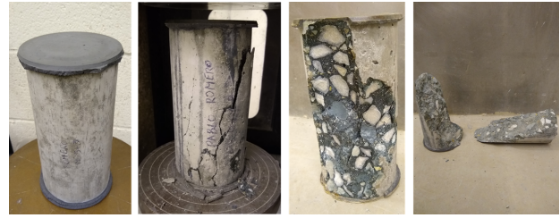
Figure 9: Photographs of some concrete cylinders made according to novel formulations, undergoing laboratory testing for compressive strength.
