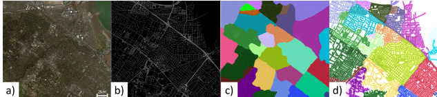
Figure 1. Street Addresses starts with (a) satellite imagery, predicts (b) roads, creates (c) regions, to obtain (d) addresses.
