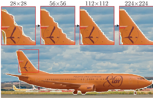
Figure 7: Anti-aliasing with PointRender. Precise object delineation requires output mask resolution to match or exceed the resolution of the input image region that the object occupies.
