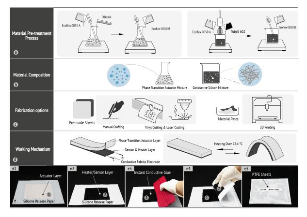
Figure 2: (a) Material preparation steps for phase transition actuator and conductive silicone; (b) The material composition; (c) The two available fabrication options: 2D cutting & 3D printing; (d) The fundamental working mechanism for the system; (e) Detailed fabrication process.
