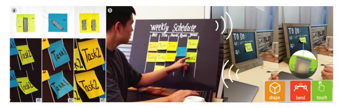
Figure 12: (a) Different actuation modalities; (b) Remotely synchronize the task progress by tapping or bending the Post-it note with PITAS attached on the back.
