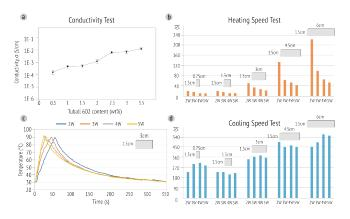
Figure 7: (a) Conductivity test results; (b) Heating speed test for five samples with different sizes; (c) Temperature curve for different input power; (d) Cooling speed test for five samples with different sizes.
