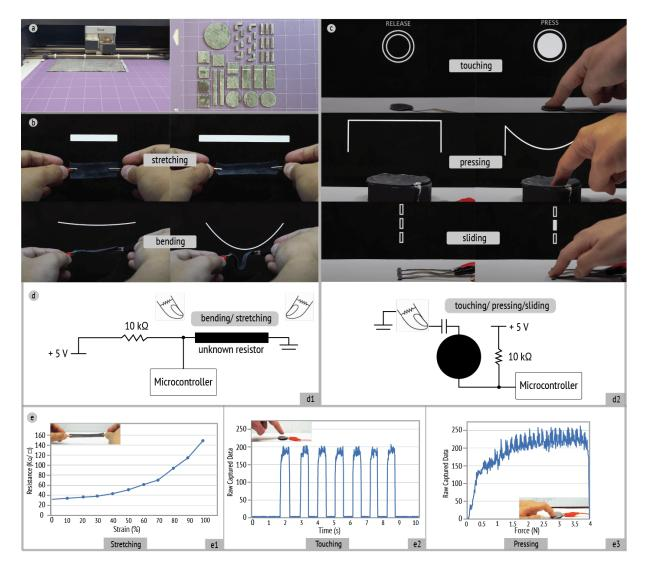
Figure 4: (a) Vinyl cutting process for the sensing samples; (b) Two example resistive sensing modalities: stretching and bending; (c) Three example capacitive sensing modalities: touching, pressing and sliding; (d) schematics for both sensing approaches; (e) Raw sensing data for resistive (stretch) sensing and capacitive (touch, press) sensing.
