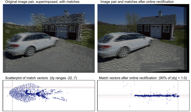
Figure 3. Online rectification example. Left: original image pair with matches overlaid, and scatterplot of match vectors, exhibiting large vertical disparities \Delta y . Right: image pair and matches after online rectification. More than 90% of |\Delta y| are below 1.0 pixels, and points at infinity are stabilized at \Delta x = 0 .
