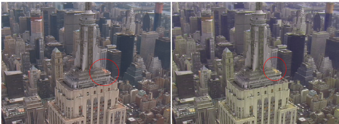
Figure 2 Left video frame is output of SW pipeline, while right video frame is output of ASIC pipeline, wherein color may be shifted if color metadata is not handled properly by ASIC.
