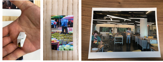
Fig. 9: Paper dolls are made by dressing up printed images with paper patches. We use dolls to observe the effects of camera distortions, and “scrumpled” patches to test against physical deformations that are not easily simulated.
