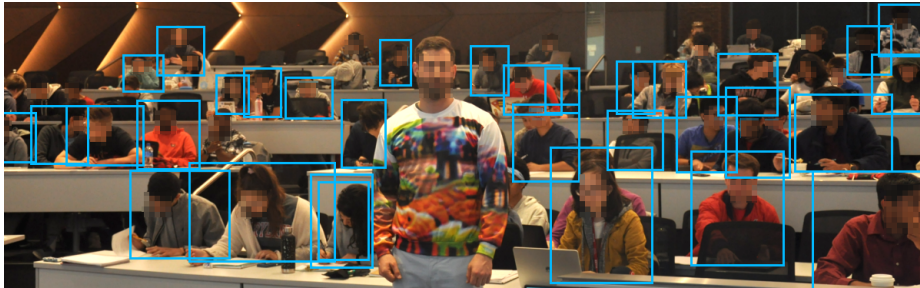
Fig. 1: In this demonstration, the YOLOv2 detector is evaded using a pattern trained on the COCO dataset with a carefully constructed objective.
