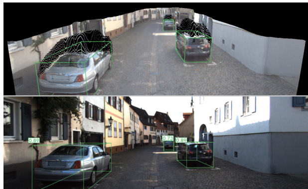
Figure 2: Example of output visualization. Top: Visualization of our predictions on the colored Pseudo-LiDAR pointcloud. Bottom: Visualization of our predictions, with corresponding confidence score, on the input RGB image.
