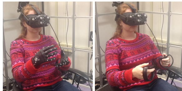
Figure 1: In our experiment, participants complete block stacking puzzles in virtual reality (left), controlling their avatar’s hands either with tracked gloves (middle, left) or with touch controllers (middle, right). The avatar’s hands are varied to fit the participant’s hands in size or to be 25% larger or smaller (right).
