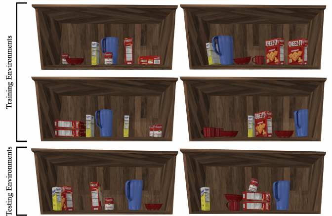
Fig. 2. For collecting our YCB-Extrinsic-Contact dataset we simulate six kitchen cabinet environments with different configurations of YCB objects in PyBullet. Four scenes are use for collecting training data and the other two for testing. Objects in these environments can move around as the robot interacts with the environment when collecting extrinsic contact data.
