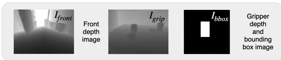
Fig. 7: Simulated and real-world visual observations. The visual observations consist of: (1) two front depth images from the robot, concatenated to make a single image I_{front} ; (2) a depth image from the gripper of the robot I_{grip} ; (3) a bounding box image around the target object, if detected by an object detector operating on the gripper camera I_{bbox} . To minimize the sim-to-real gap, we de-noise the real depth images using a fast depth completion algorithm that leverages classical image processing [43].
