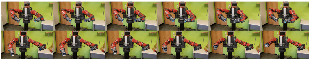
Figure 4: Depiction of execution of the learned primitives on real world Baxter robot. Each row is a single primitive, while columns show progress of the primitive over time. Row 1 depicts a left handed reaching primitive, while row 2 shows a right handed returning primitive. More visualizations provided in supplementary material, and videos are provided in the webpage.
