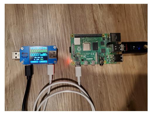
Figure 3. Energy monitoring setup.
