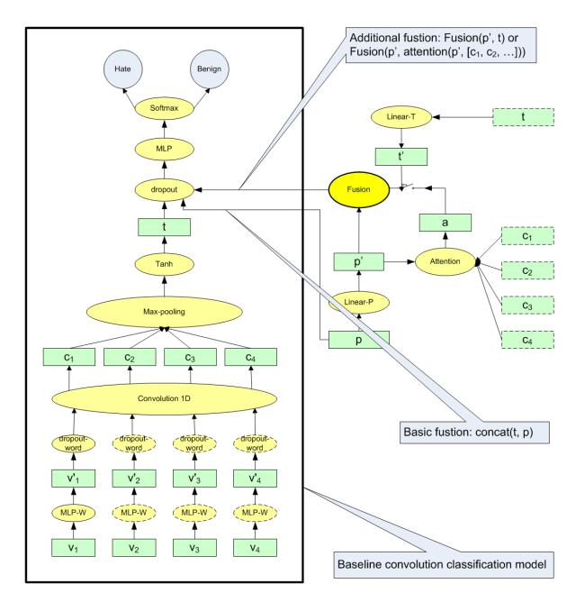
Figure 1: Model architecture of text and photo fusion: ellipses (in yellow) represent operations; and rectangles (in green) represent vectors. Shapes in dot lines are *clones* of their corresponding components.
