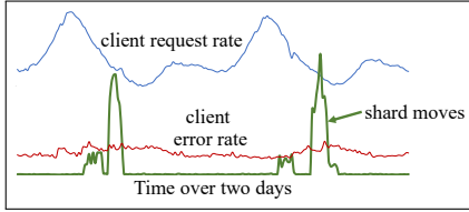
Figure 18. (Production) No increase in client errors during upgrades, thanks to graceful shard migration.
