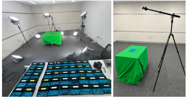
Figure S1. Our setup for capturing the Eyeglasses dataset.
