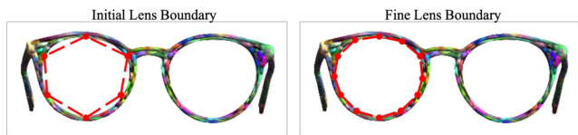
Figure S7. Lens boundary estimation. We demonstrate how the coarse boundary from glasses key points is refined to a finer lens boundary. Left is the six key points detected from images. Right is the fine lens boundary after one subdivision. In our experiments, we repeat the proposed subdivision three times.
