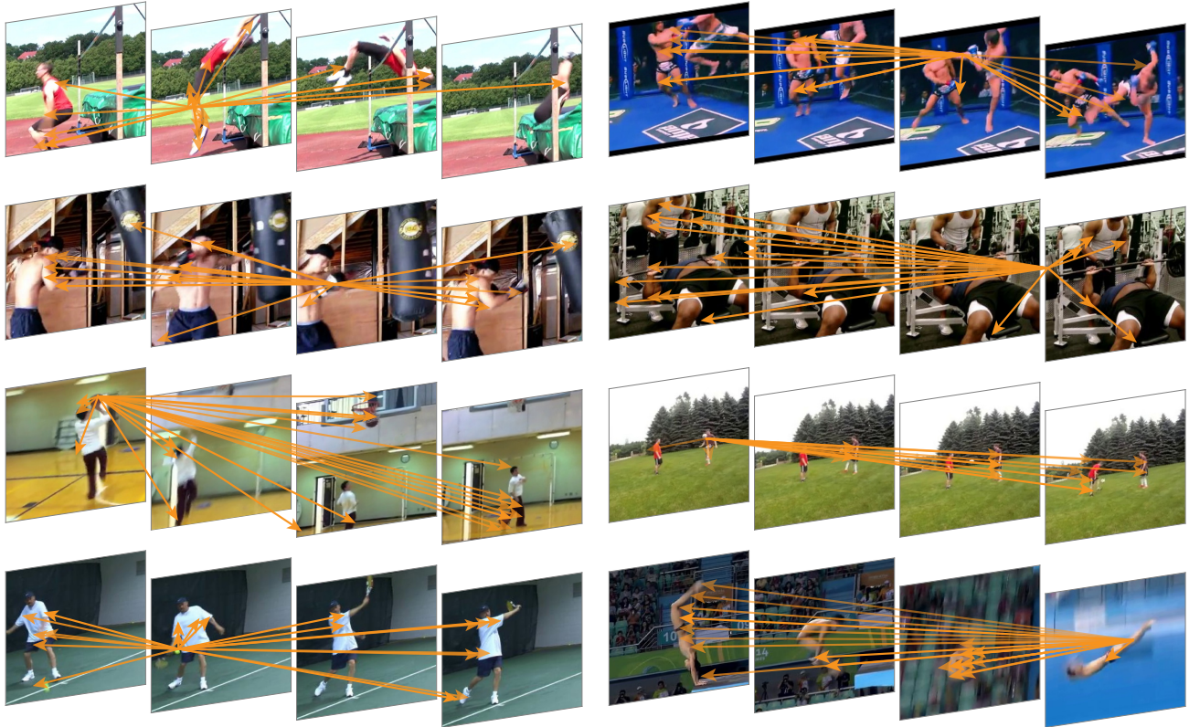
Figure 3. Examples of the behavior of a non-local block in \text{res}_3 computed by a 5-block non-local model trained on Kinetics. These examples are from held-out validation videos. The starting point of arrows represents one x_i , and the ending points represent x_j . The 20 highest weighted arrows for each x_i are visualized. The 4 frames are from a 32-frame input, shown with a stride of 8 frames. These visualizations show how the model finds related clues to support its prediction.
