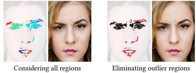
Fig. 5. Outlier detection. Left: Considering all the regions with significant ratio values (each connected component is colored in a unique color) yields the expressive image on the left. Right: By eliminating the outlier regions (highlighted in red), we obtain a refined result, which does not contain, for example, the cast shadow beside the nose. ©Unsplash photographer Seth Doyle.
