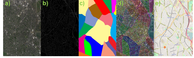
Figure 8. Stages of a generative map of a US city. We show (a) the input satellite image tile, (b) the extracted roads, (c) the created regions, and (d) the generated map, comparing to (e) the OSM of the same area. (zoom in for details)
