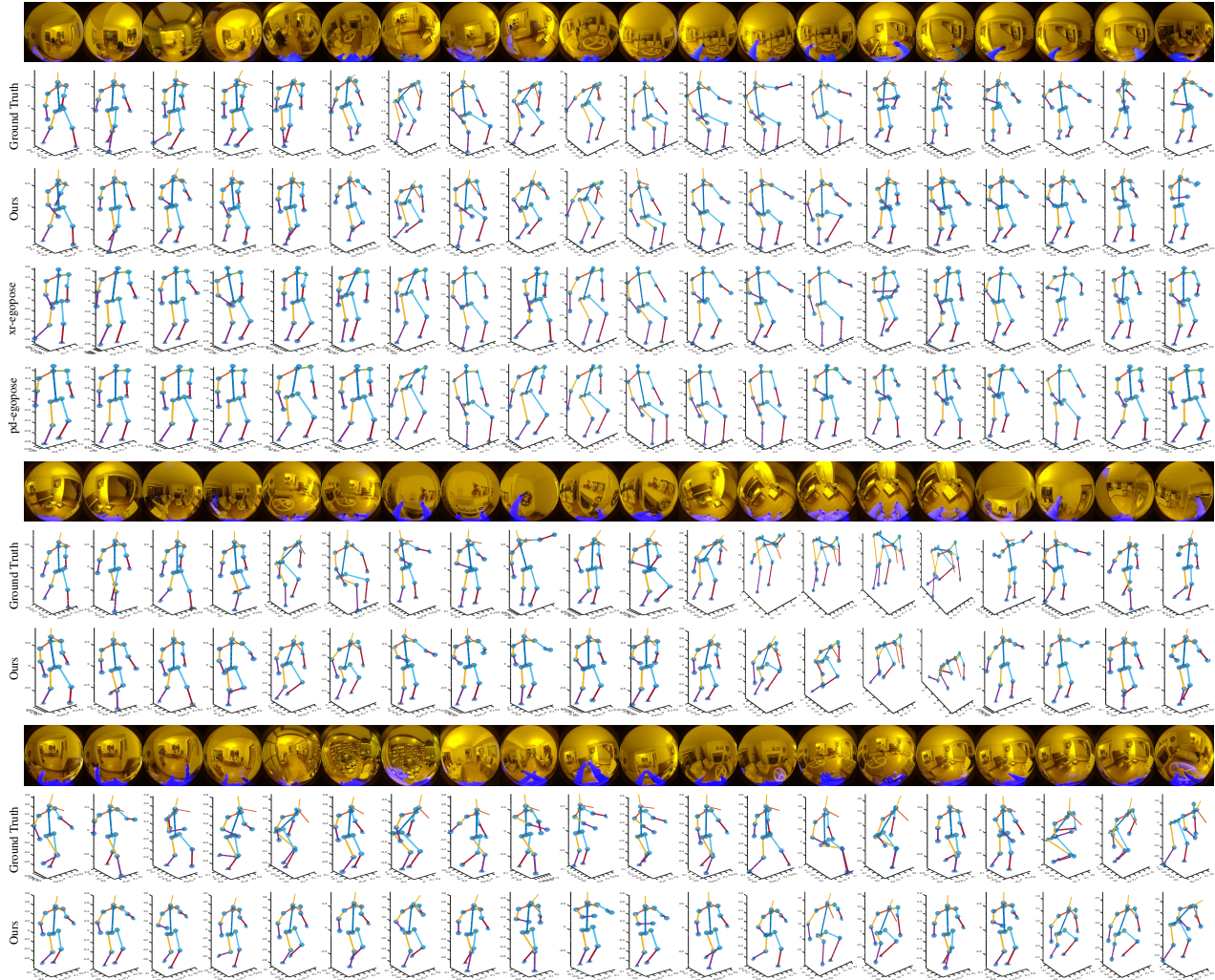
Figure 12. Real video test. Rows 1,6,9: body shape segmentation overlaid on the egocentric video. Rows 2,7,10: ground truth egoposes. Rows 3,8,11: the proposed method’s (ours III) results. Row 4: xr-egopose II result. Row 5: pd-egopose result. (Best viewed in color).
