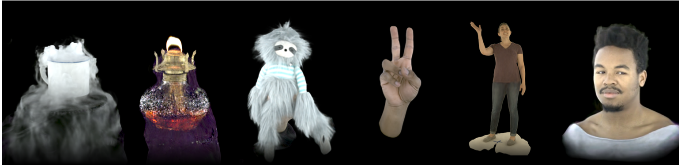
Fig. 1. Renderings of objects captured and modeled by our system. The input to our method consists of synchronized and calibrated multi-view video. We build a dynamic, volumetric representation of the scene by training an encoder-decoder network end-to-end using a differentiable ray marching algorithm.
