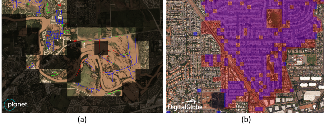
Figure 2: (a) Use DII to infer severe flooding damage areas (highlighted) during Hurricane Harvey, based on changes in detected roads (Blue: true positive, Green: false positive, Red: false negative); (b) Use DII to infer severe fire damage areas at Santa Rosa, based on changes in detected buildings (Blue), compared with shapefile of fire damage area obtained from FRAP [1] (Red)
