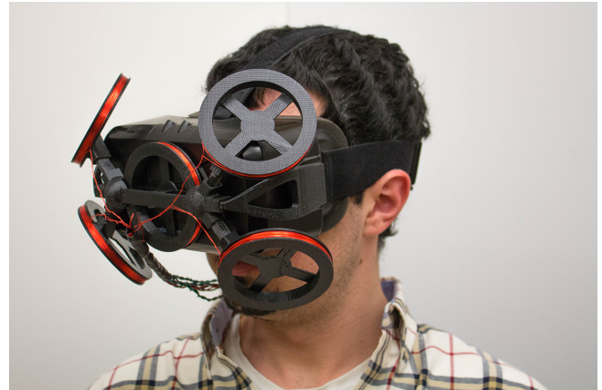
Figure 1. The EyeContact scleral coil tracker can clip to an HMD and does not require the use of a head mount or room-sized field coils
