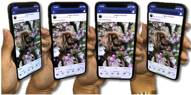
Fig. 11. Rotating phone induces parallax through sensing from the gyro.
