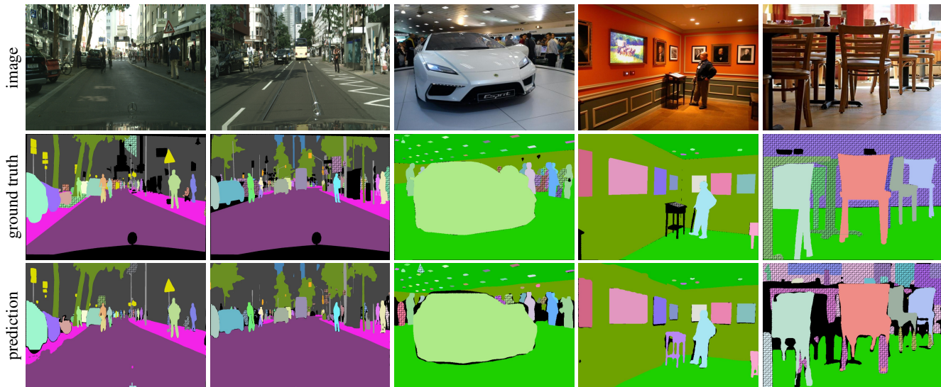
Figure 9: Panoptic segmentation results on Cityscapes (left two) and ADE20k (right three). Predictions are based on the merged outputs of state-of-the-art instance and semantic segmentation algorithms (see Tables 3 and 4). Colors for matched segments (IoU>0.5) match (crosshatch pattern indicates unmatched regions and black indicates unlabeled regions). Best viewed in color and with zoom.
