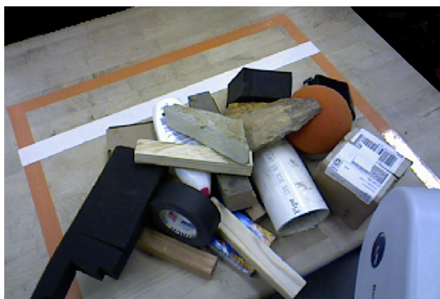
Fig. 1 Perceiving and manipulating unknown objects in a pile: Each detected object has a set of affordances (pushing, pulling or grasping). The robot selects the best next interaction for clearing the pile of unknown objects. The orange boundaries mark reachable space. The robot cannot grasp an object behind the white boundary , but may push or pull on it
