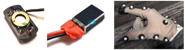
Fig. 8. A voice coil actuator (Tectonic TEAX14C02-8) and linear resonance actuator (KOTL LV111738) used to evaluate our system. Right shows a pose-tracked mesh glove with the LRA mounted to the index fingertip.
