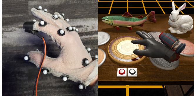
Fig. 1. A tracked glove with a vibrotactile actuator (left) allows us to interact with virtual objects and feel textured surfaces (right) with haptic and audio feedback synthesized using methods described in this work.
