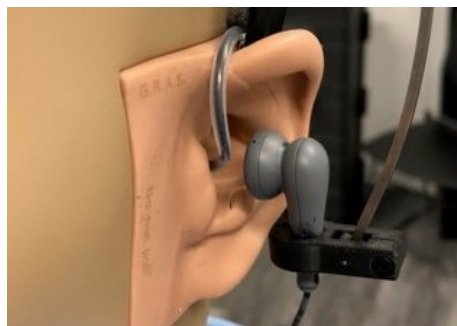
Fig. 1: Custom “floating” headphones (Sennheiser MX475) and binaural microphones (Brüel and Kjær 4101-B) mounted on KEMAR head and torso simulator (GRAS).
