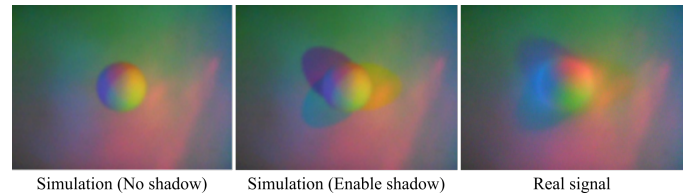
Fig. 8: TACTO supports rendering shadows to obtain more realistic simulations. The real-world measurement is collected from a DIGIT sensor touching a ball of 3.7 mm diameter.
