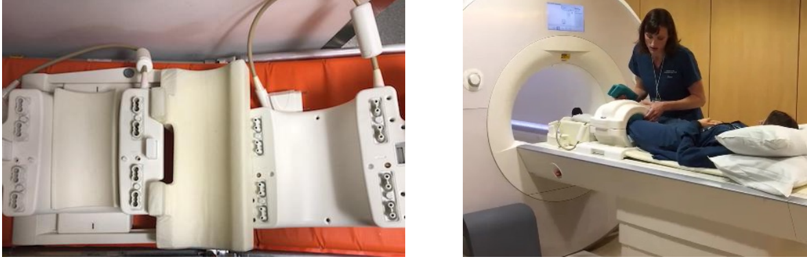
Figure 1: The receiver coil housing and its positioning on a patient for a knee MR examination.
