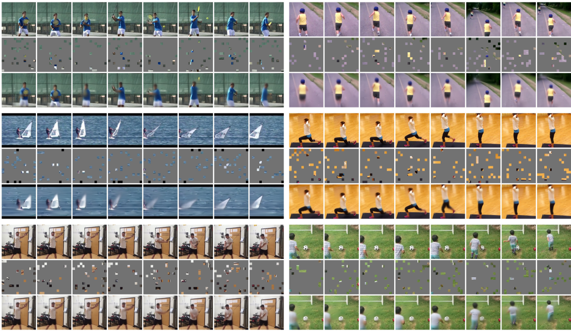
Figure 2: Visualizations on the Kinetics-400 [35] validation set (masking ratio 90% ). We show the original video (top), masked video (middle), and MAE output (bottom) for each sample. This model reconstructs the original pixels. The video size is 16 \times 224 \times 224 and the spacetime patch size is 2 \times 16 \times 16 (the temporal patch size of 2 is not visualized here). Each sample has 8 \times 14 \times 14 = 1568 tokens with 156 being visible. For better visualizations, the known patches in the output are from the original input. Fig. 7 shows more examples.
