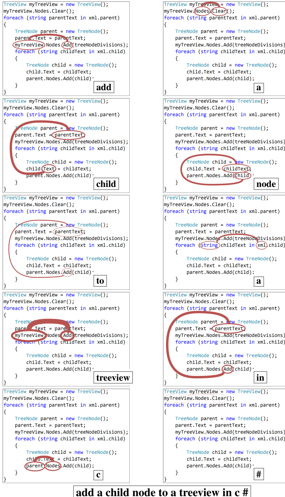
Figure 5: Example of code captioning for a C# code snippet from our test set. The text boxes at the bottom of each figure are the predictions produced by our model at each decoding step. The highlighted paths in each figure are the top-attended paths in each decoding step, and their widths are proportional to their attention weight (because of space limitations we included only the top-attended path for each decoding step, but hundreds of paths are attended at each step).
