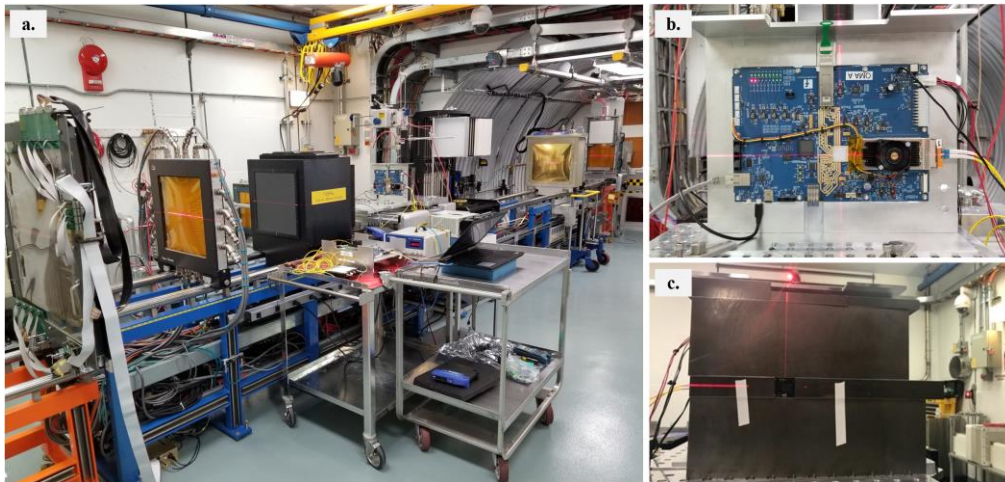
Figure 4. Heavy ion radiation test setup at NSRL. (a) The OMA fixed to a test stand in line of heavy ion beam and (b) the DUT aligned to center of the heavy ion beam path using lasers. (c). Lead blocks used to shield the rest of the OMA from heavy ion radiation.
