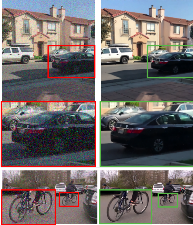
(b) Sample EVRNet results on unseen videos. Left: compressed and noisy frames. Right: Restored frames.
