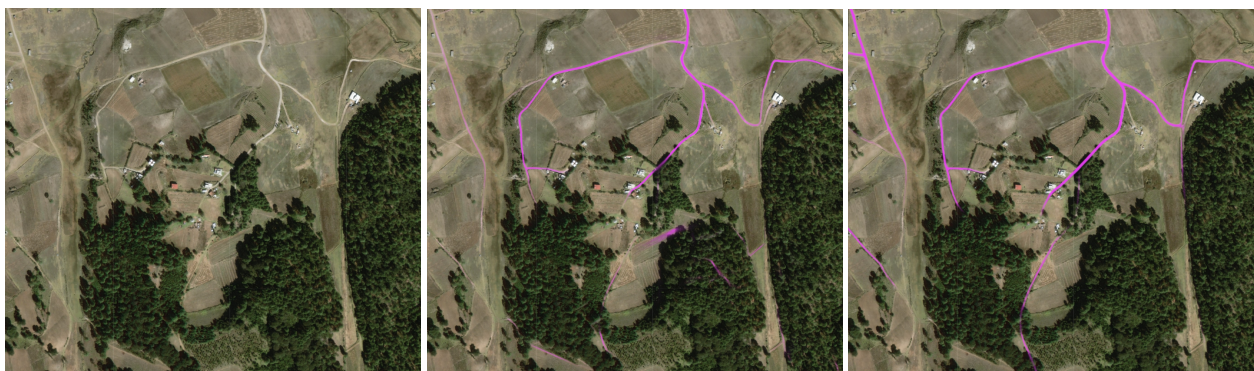
Figure 4. Road extraction from satellite imagery in rural Mexico. Left: Satellite Imagery. Middle: THA/IND/IDN trained model. Right: Global OSM trained model. The model trained on DeepGlobe data misses the road in the top left almost entirely and leaves several roads in the middle of dense trees whereas the globally trained model performs well.
