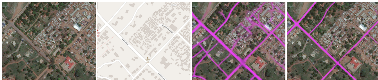
Figure 5. Road extraction from a relatively well mapped area in Kampala, Uganda. From left to right: satellite imagery, OSM(manually mapped), THA/IND/IDN trained model, Global OSM trained model. The model trained on DeepGlobe draws numerous non-existent roads through the middle of houses whereas the globally trained model performs well.
