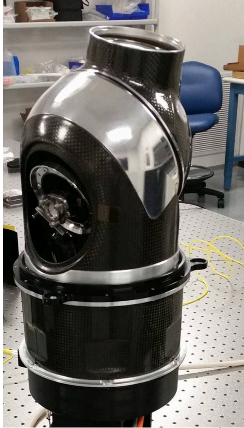
Figure 8: Operational prototype gimbal complete with motors, encoders and optics.
