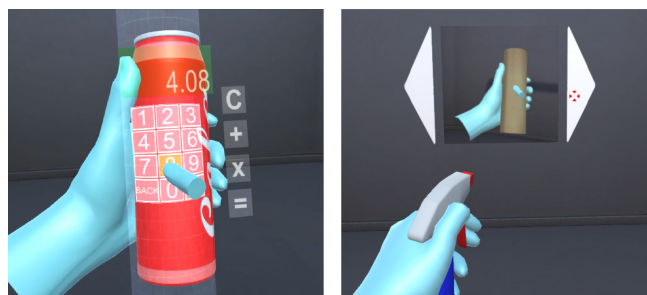
Figure 15. Left: On objects with smaller surface area, buttons can be split between the surface and midair. Knowing where the hand is, the midair overflow buttons can be placed to the side of the hand. Right: The spray bottle can be used as a virtual pointing, using the hand orientation to point and the trigger gesture to select.
