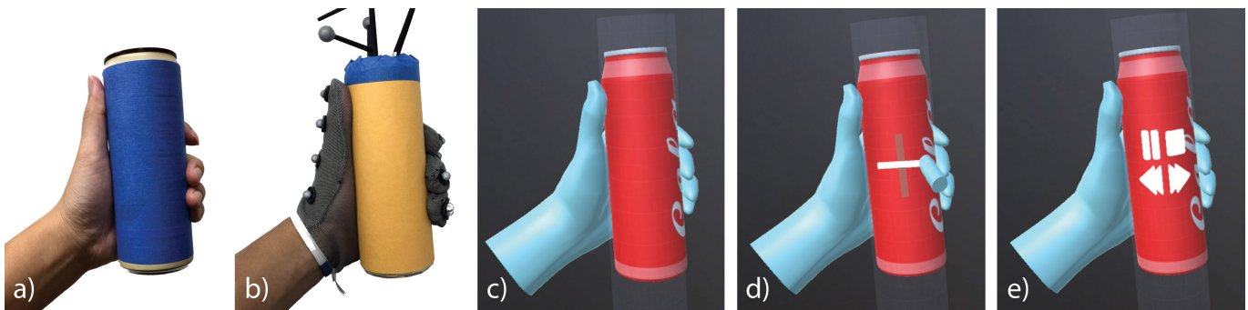
Figure 1. Gripmarks explore the concept of transforming an object a user is already holding, such as a soda can (a), into an input surface for mixed reality by recognizing the grip through hand tracking (b). The object is tracked only for visualization purposes and represents a real object in simulated augmented reality. The grip is recognized as a cylinder grip and the surface of the cylindrical object is estimated (c). The user employs an activation gesture on the estimated surface (d) to specify the size and location of a simple interface, such as a media player (e).
