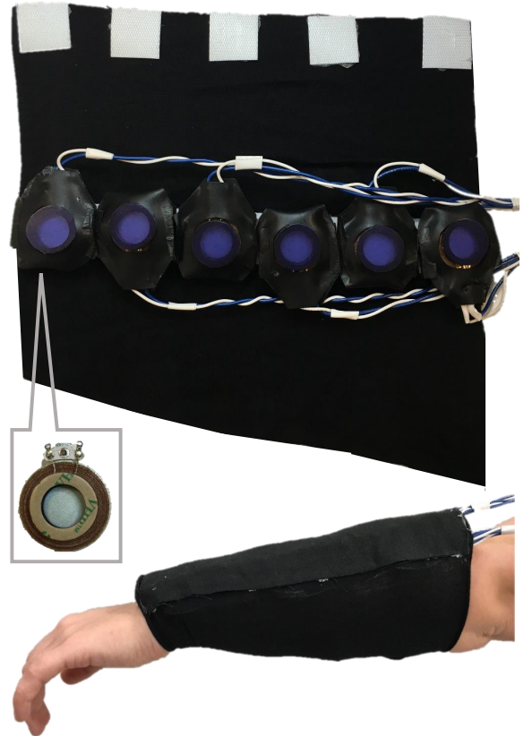
Fig. 1. Device for creating the sensation of continuous lateral motion using sequential indentation. A linear array of voice coils are controlled to apply a pre-determined indentation profile to the arm.
