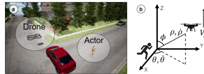
Fig. 2: Experimental setup: a) Photo-realistic simulator with an animated character and aerial vehicle; b) Shot parameters that define the vehicle’s position relative to the actor, in spherical coordinates.
