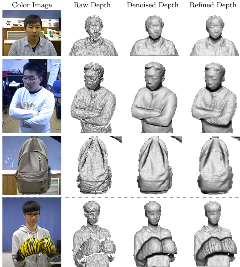
Fig. 5. Qualitative results on validation set. From left to right in each row: aligned RGB image, raw depth map, output of our denoising net D_{dn} and output of our refinement net D_{dt} with added high-frequency details. D_{dn} captures the low-dimensional geometry without noise, D_{dt} shows fine-grained details. Although trained on human body dataset, our model also produce high-quality depth map on general objects in arbitrary scenes, eg. the backpack sequence. The last row shows typical failure case of our network, which may suffer from non-Lambertian reflectance.
