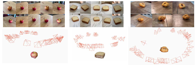
Figure 3: In order to study learning 3D object categories in the wild, we crowd-sourced a large collection of object-centric videos from Amazon Mechanical Turk. The top row shows frames from three example videos, the bottom two rows show SfM reconstructions of the videos together with tracked cameras.
