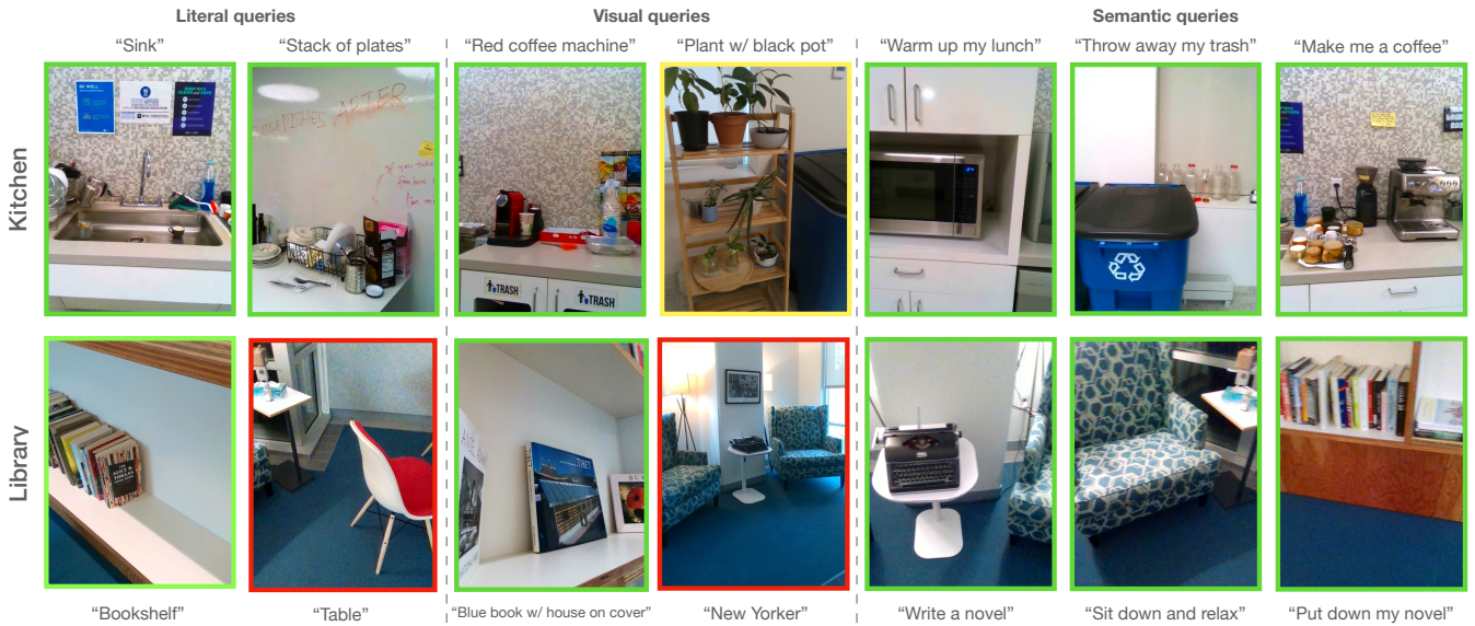
Fig. 8: Examples of the robot’s semantic navigation in two different testing environments, looking at objects given different queries. The images show the robot’s POV given the associated query, with color coded borders showing approximate correctness. The rows show different two different scenes, top being in a lab kitchen and the bottom in our lab’s library/lounge space, shown in detail in figure 7.
