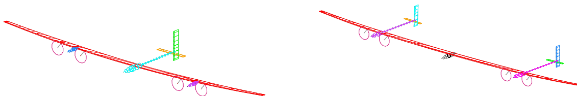
Figure 1. Typical aircraft configurations analysed using this framework (left: single-boom, right: dual-boom)
