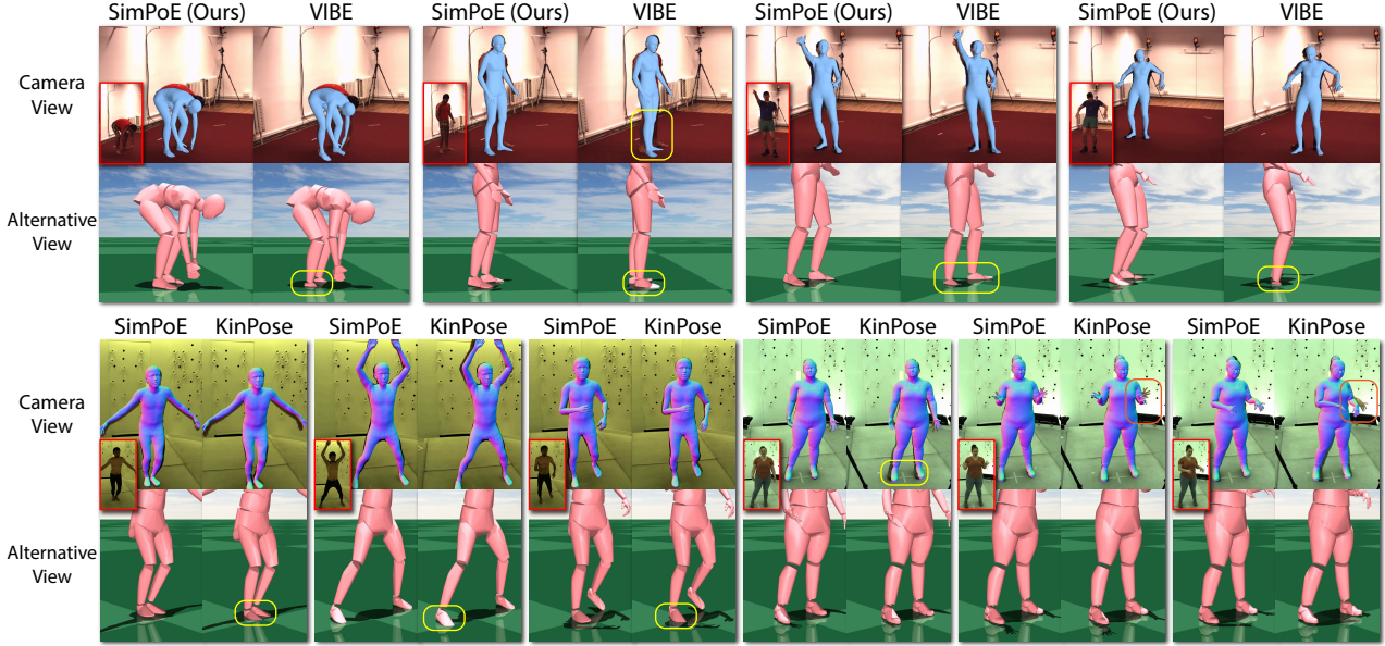
Figure 3. Visualization of estimated poses in the camera view and an alternative view. SimPoE estimates more accurate poses and foot contact. Pose mismatch and ground penetration are highlighted with boxes. Please see the supplementary video for more comparisons.
