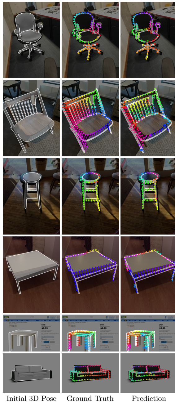
Fig. 13: Additional qualitative examples of our predicted geometric correspondence fields. Our predicted 2D displacement vectors are highly accurate for many different objects and scales. Best viewed in digital zoom .
