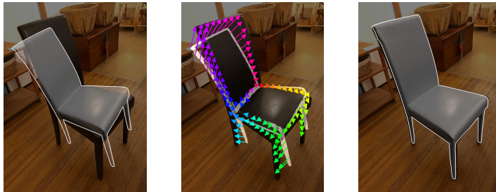
Fig. 1: Given an initial 3D pose predicted by a feed-forward network ( left ), we predict deep cross-domain correspondences between real-world RGB images and synthetic 3D model renderings in the form of geometric correspondence fields ( middle ) that enable us to refine the 3D pose in a differentiable rendering framework ( right ).
